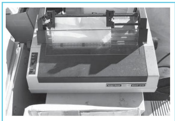
*Fig. 2.2.3: Daisy-Wheel Printer*
